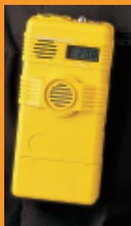
Furmanite pipe freezing procedures specify the use of personal oxygen monitors
